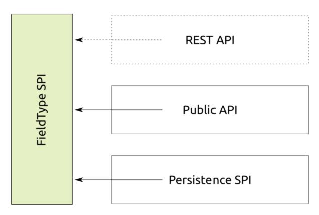
On the top layer, the FieldType needs to provide conversion from and to a simple PHP hash value to support the REST API. The generated hash value may only consist of scalar values and hashes. It must not contain objects or arrays with numerical indexes that aren't sequential and/or don't start with zero.
