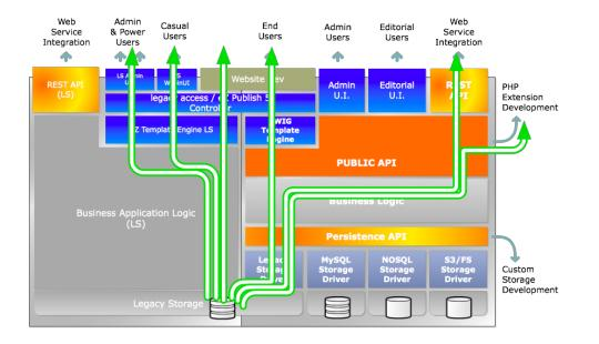
In this model, the two kernels can be used and the system can this way benefit from the Public API and the new REST API built on top.
