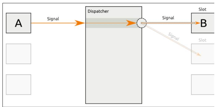
In the shown schematics, object B and one other object are interested in a certain signal. B is a so-called Slot that can be announced to be interested in receiving a Signal (indicated by the circular connector to the dispatcher). Object A now sends the corresponding Signal. The Dispatcher takes care of realizing the dependency and informs the Slot A (and one other Slot) about the occurrence of the Signal.
