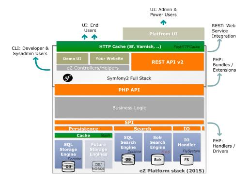
The architecture is layered and uses clearly defined APIs between the layers.
