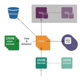
This diagram illustrates how clustering of eZ Platform is typically set up, the parts illustrate the different roles needed for a successful cluster setup. The number of web servers, Memcached servers, Solr servers, Varnish servers, Database servers, NFS servers, as well as whether some servers play several of these roles (*typically running Memcached across the web server*) is up to you and your performance needs.
